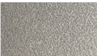
55% Al-Zn Alloy Coated Steel with Acrylic Coating (97)
